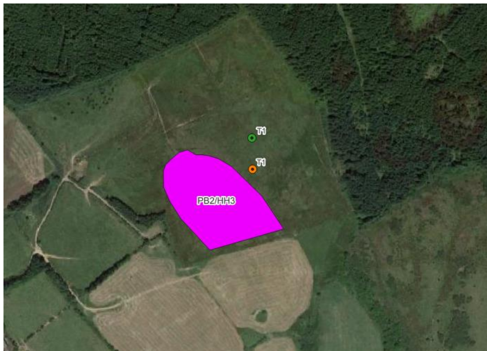
Figure 4-10: Iteration 3 – Relocation of T1 – Increase distance from area of Upland Bog/Wet Heath
