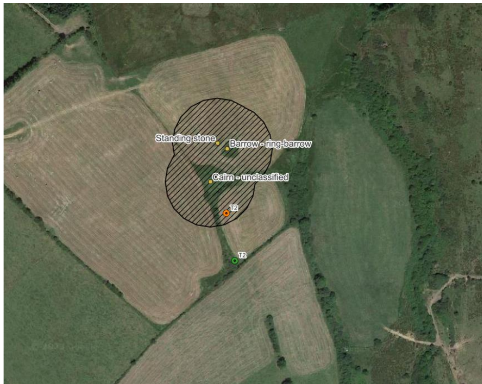
Figure 4-11: Iteration 4 – Relocation of T2 - Increase distance from Archaeological Features
