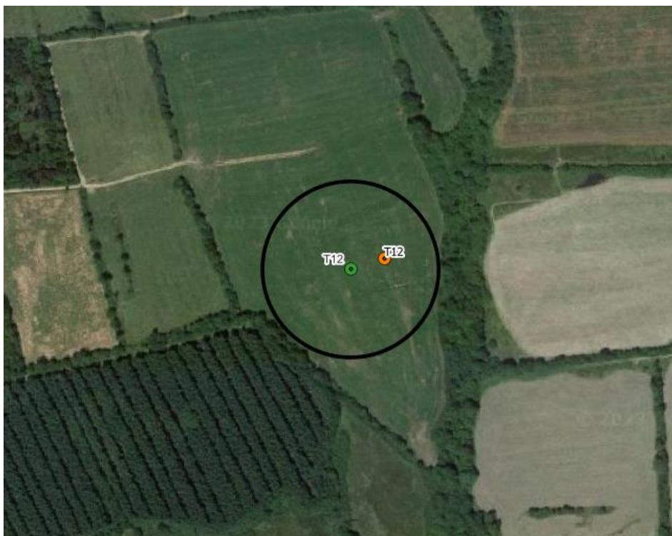
Figure 4-12: Iteration 5 - Relocation of T12 to Avoid Felling of Woodland
